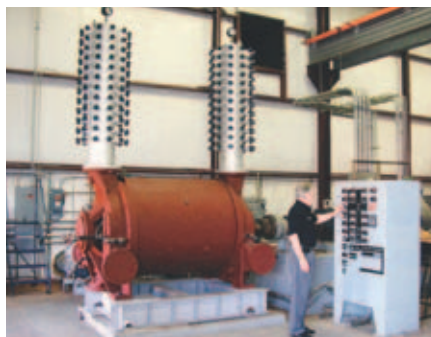
A Vooner FloGard two-inlet cone port pump tested in the Charlotte, NC test facility
