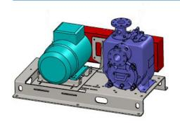
In this version, the motor is connected to the pump by means of a V-belt transmission. By varying the gear ratio, the exact pump speed can be set. The motor can be optionally placed on the left or right hand side of the pump.
