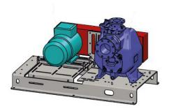
In this version, the motor is connected to the pump by means of a V-belt transmission. By varying the gear ratio, the exact pump speed can be set. The motor can be optionally placed on the left or right hand side of the pump.
